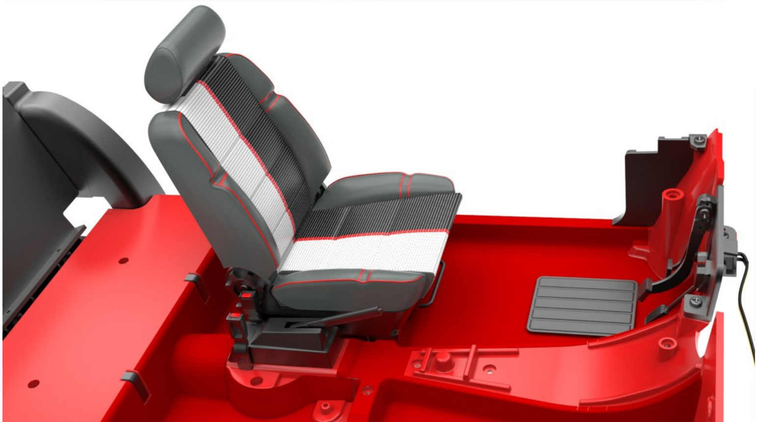
Front left seat installed .
