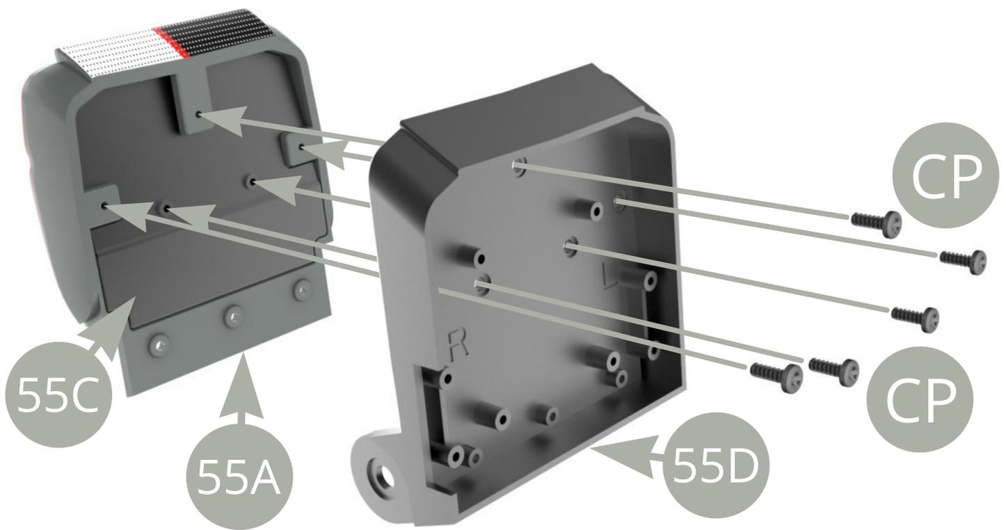
Fit **55D Front right seat base** to **55A Front right seat cushion** with **55C Cushion panel** , and fix to the latter with five **CP screws** .
