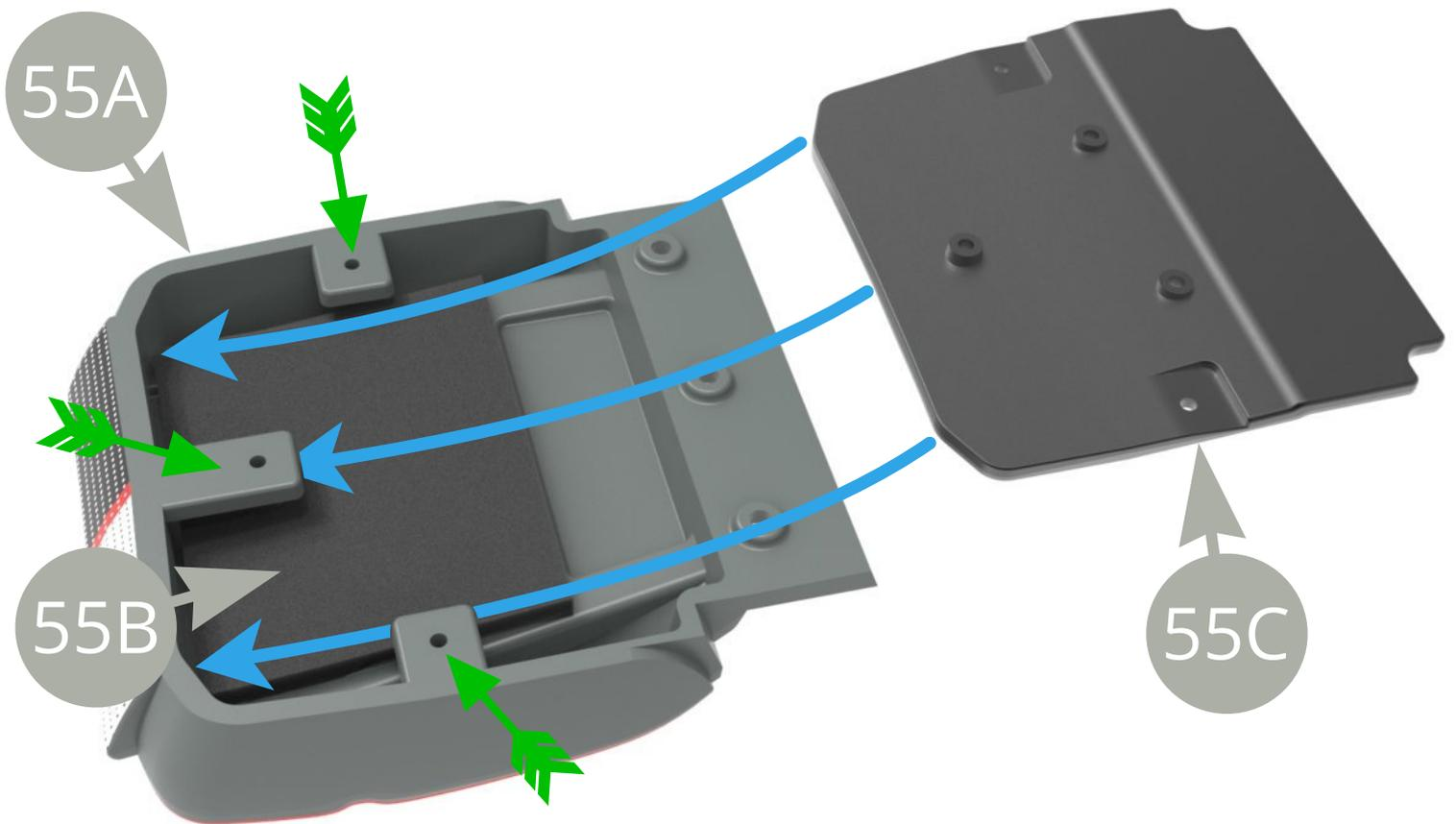
Slide **55C Cushion panel** into **55A Front right seat cushion** , on top of **55B Cushion padding** and under three tabs pointed by **green arrows** .
