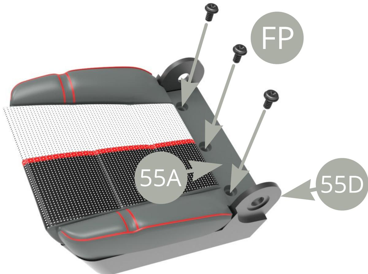
Fix **55A Front right seat cushion** to **55D Front right seat base** with three **FP screws** .
